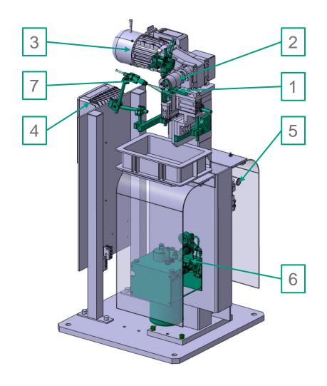
The FFT Roller Cleaning Device automatically cleans the hemming rollers without interrupting the automatic cell operation.
